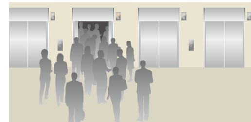
If a fully loaded car leaves a floor, a hall call is registered automatically.
